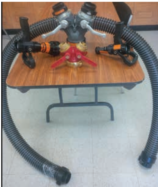
the equipment items purchased so far by NFRA. One suction hose, two Hose nozzles and two gated hose wyes.
