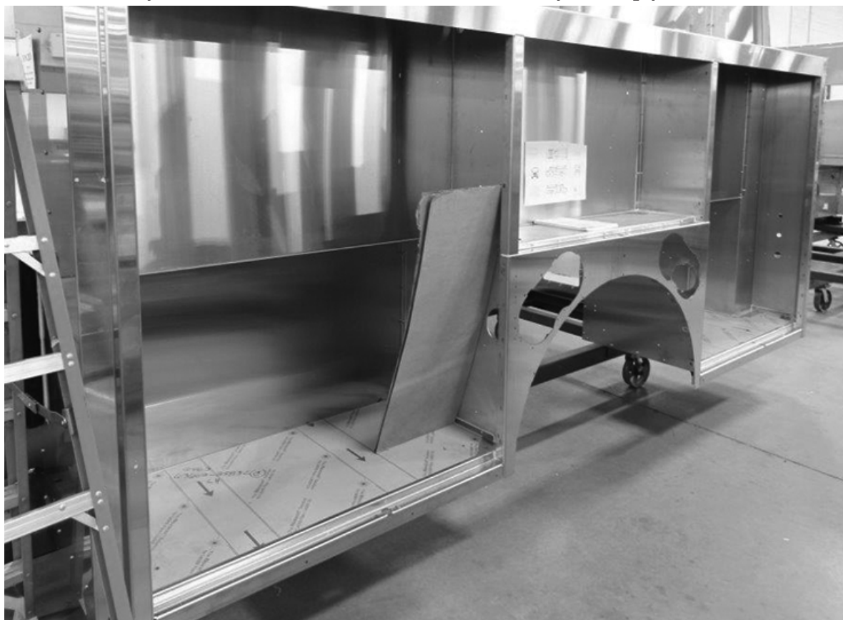
New fire pumper body under construction
